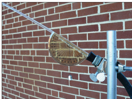
Fig. 3. The water leaves the glass tube at a launch angle of 35^\circ to the horizontal.
