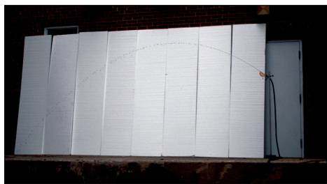
Fig. 2. Our water hose trajectory. We placed white boards behind the water stream so that the stream is more visible. The water leaves the tube 1.30 m above the ground with an initial velocity that is 35^\circ above the horizontal. The water lands 3.66 m horizontally from the base of the support rod.
