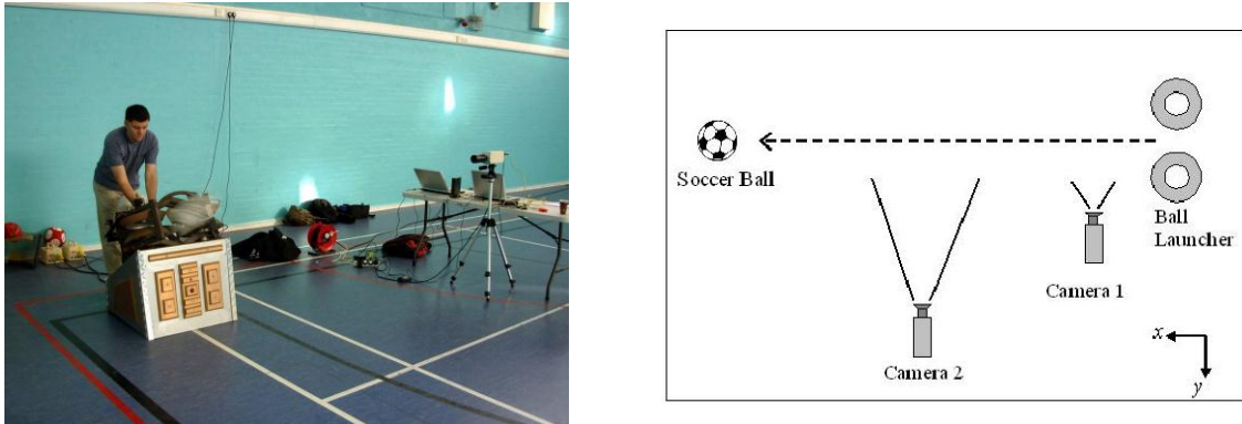
Fig. 1. (a) Our ball launcher projects a soccer ball; (b) Schematic of our experimental setup
