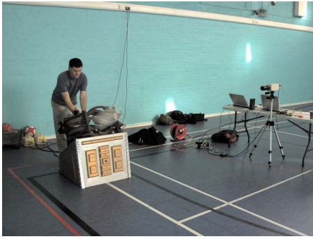
Fig. 1. Ball launcher used for the trajectory experiments. Note the ball emerging from the launcher and the location of camera 1 on the right side of the photo.
