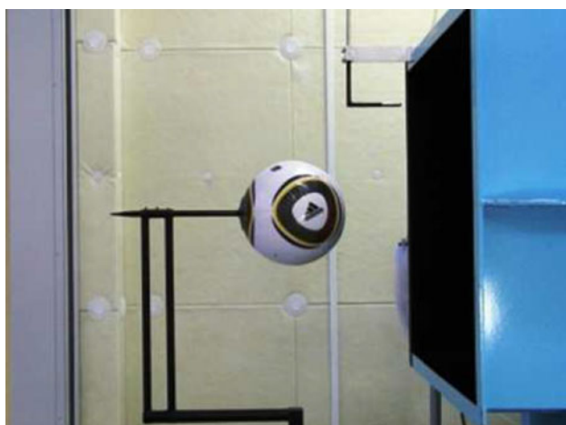
Fig. 11 Wind-tunnel set up for a Jabulani ball in a Japanese experiment (Asai T, private communication)
